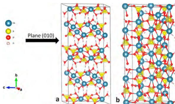
**Figure 3.** Calcium sulfate structure. (a) In gypsum (CaSO<sub>4</sub>·2H<sub>2</sub>O), the water molecules forming the plane (010) are seen. (b) In bassanite (CaSO<sub>4</sub>·<sup>1</sup>/<sub>2</sub>H<sub>2</sub>O), the water molecules reorganize and form channels.
