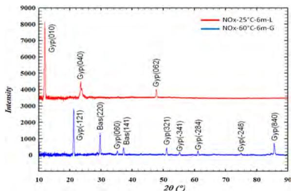
**Figure 9.** GI-XRD patterns integrated from a two-dimensional measurement of one sample with no bassanite signals (red), and another sample with gypsum (Gyp) and bassanite (Bas).
