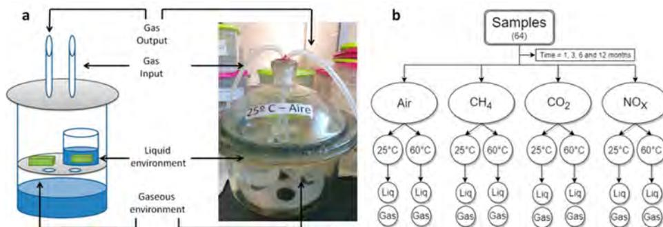
**Figure 5.** (a) Reactor configuration and (b) general planning of the microclimatic simulation.
