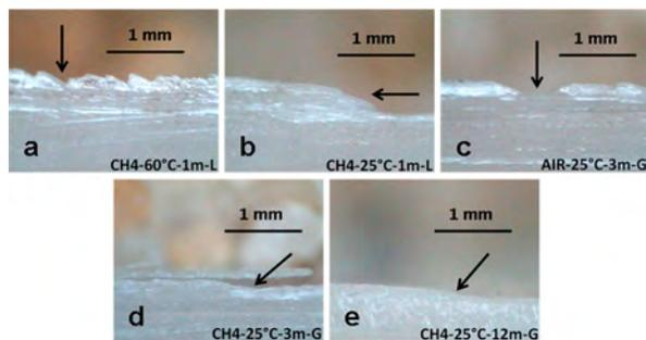
**Figure 7.** Types of surface damage detected by stereomicroscopy. (a) Irregular.  $\text{CH}_4$  at 60 °C for 1 month in liquid. (b) Slope.  $\text{CH}_4$  at 25 °C for 1 month in liquid (c) Well. Air at 25 °C for 3 months in gas. (d) Detachment.  $\text{CH}_4$  at 25 °C for 3 months in gas. (e) Minor slope.  $\text{CH}_4$  at 25 °C for 12 months in gas.
