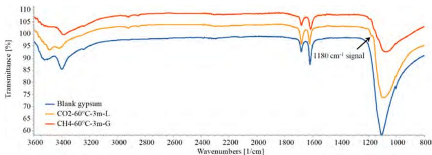
Figure 8. IR spectra for selected samples: (blue) blank gypsum sample; (orange) sample with the characteristic 1180 cm<sup>-1</sup> signal; and (red) sample with a signal below the detection limit. Bassanite was identified in combination with gypsum signals.
