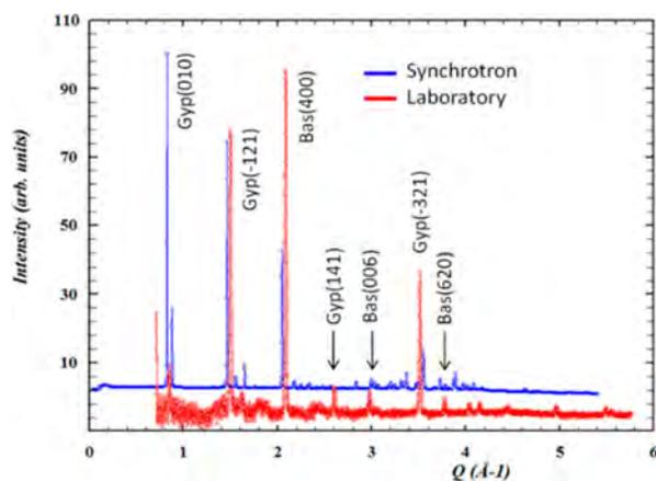
**Figure 10.** Comparison of laboratory and synchrotron XRD patterns of a bassanite-containing sample. Gypsum and bassanite peaks are identified for the CH<sub>4</sub>-25°C-3m-G sample.
