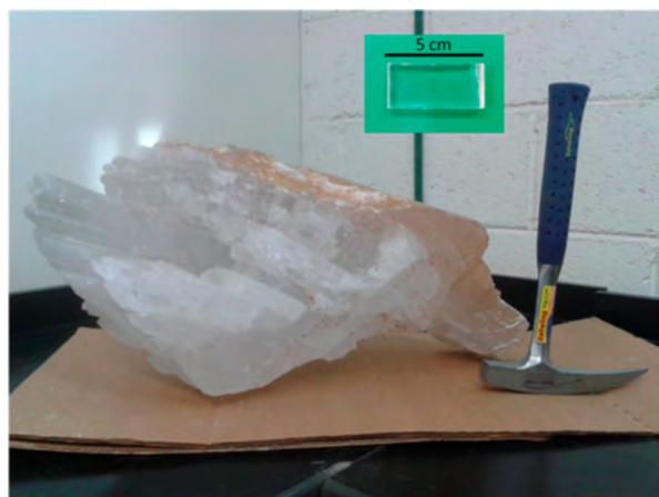
**Figure 4.** Bulk specimen from Giant Crystals Cave. In the green box, a sample as used in the experimentation can be seen.
