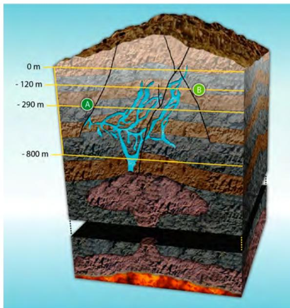
**Figure 1.** Naica mine cross section. Magmatic intrusion is shown in red; blue lines describe the mineralization. (A) Cave of Crystals and (B) Cave of Swords locations. Adapted with permission from García-Ruiz, J. M.; et al. *Geology* 2007, 35 (4), 327–330. Copyright 2007 The Geological Society of America.
