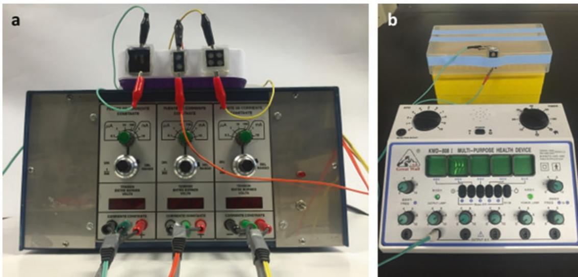
**Fig. 4** Two pieces of apparatus used for e-crystallization of proteins: (a) for applying DC ranging from 2–6  $\mu\text{A}$ , (b) for applying AC during the crystallization of proteins. First, nucleation is induced and then the crystal growth proceeds via vapor diffusion
