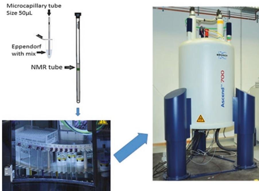
**Fig. 6** A setup for experiments performed in the presence of strong magnetic field. Two types of capillaries are used: glass pipettes and NMR tubes. The magnetic field should be applied from 500 to 700 MHz (11.7–16.5 T) by using an NMR apparatus, this is that commonly used in analytical chemistry laboratories
