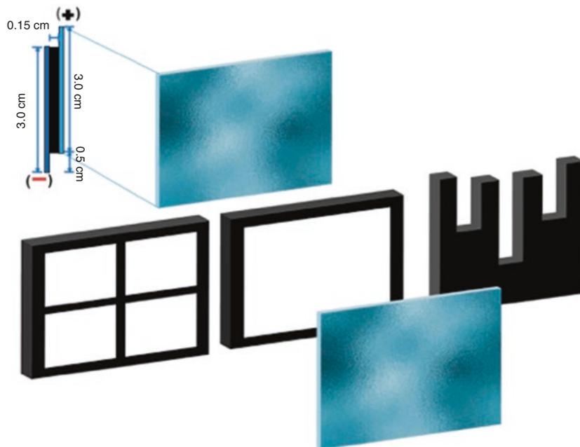
**Fig. 3** Different designs of e-crystallization growth-cell for applying electric field to the crystallization process of biological macromolecules. The two frames on the *left* are useful for batch crystallization setup, and the one on the *right* is for a vapor diffusion setup
