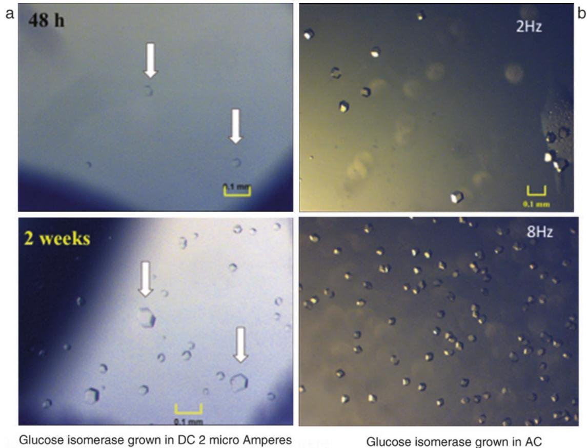
**Fig. 5** Crystals of glucose isomerase grown: (a) when a direct current (DC) of 2  $\mu\text{A}$  is applied for 48 h and subsequently the crystal growth proceeds in 2 weeks by the sitting-drop setup, and (b) when an alternant current (AC) of 2 and 8 Hz is applied for 48 h. The bar scale for (b) is the same at 2 and 8 Hz
