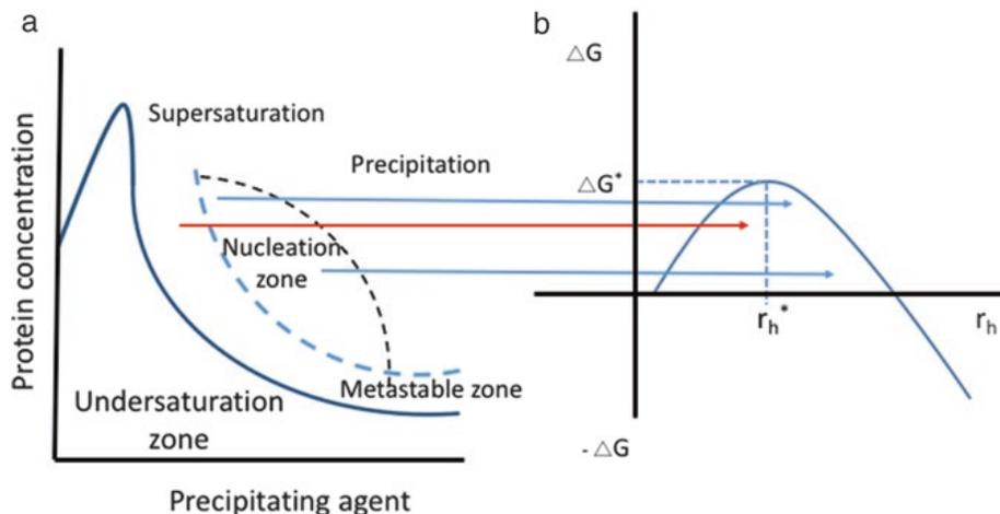
**Fig. 2** (a) The solubility phase diagram (also known as Oswald-Miers diagram) is divided into different zones: undersaturated, supersaturated, metastable, nucleation, and precipitation. (b) The energetics of the system is very important to understand; it expresses the kinetics of the crystallization and allows to predict the critical size of the nucleus to be converted into crystal
